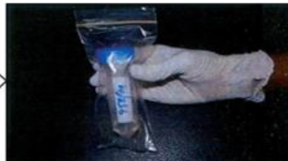
Step 4: Insert the tube to the Zip lock poly bag and close properly
